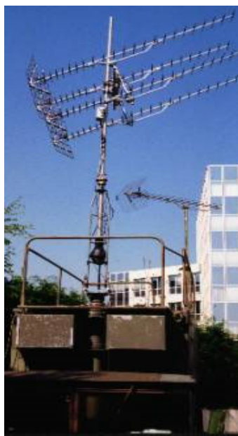
TV-radar with Video carrier and line sync. Pulses, Thales patent
