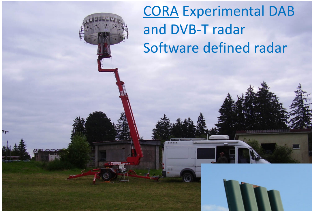
PETRA II : Passive Experimental Tv RAdar
