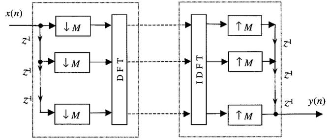
Fig. 4. Block diagram of a DFT filter bank.
