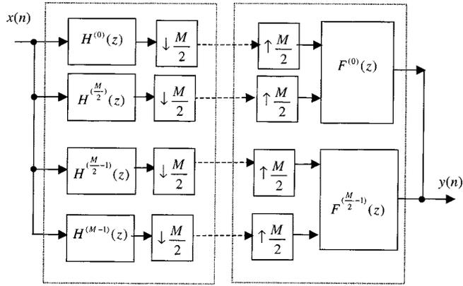
Fig. 8. Block diagram of a modified QMF bank.
