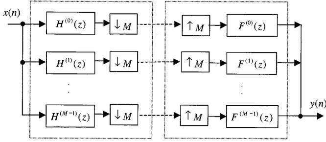
Fig. 3. Block diagram of a filter bank.
