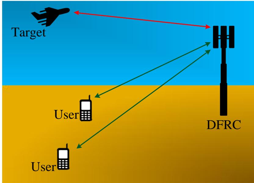
Figure 1: The principle of dual-function radar-communications.
