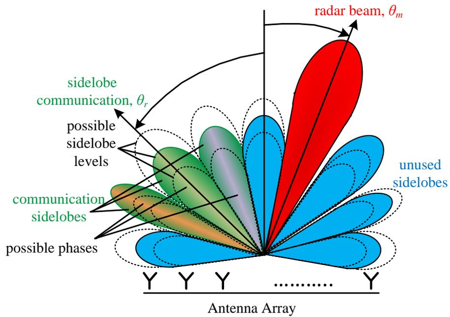
Figure 2: The proposed DFRC strategy using QAM-based sidelobe modulation.
