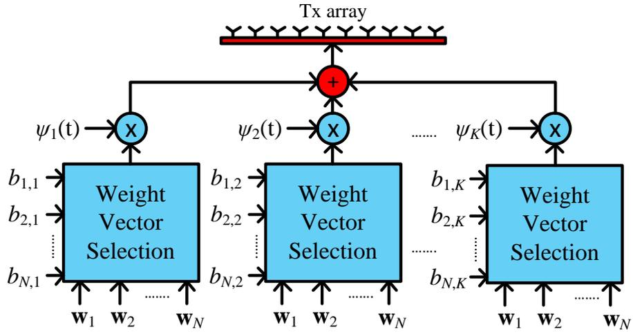
Figure 3: The proposed QAM-based DFRC approach using QAM-based sidelobe modulation (coefficients  $b_{n,k}$  are the function of  $\tau$ ).
