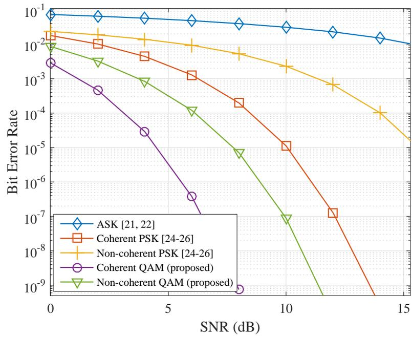
Figure 7: Bit error rate comparison for the multi-waveform ASK-based method [21, 22], multi-waveform PSK-based method (coherent and non-coherent case) [24–26] and the proposed QAM-based method (coherent and non-coherent case).
