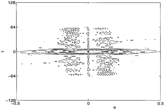
Fig. 3. Ambiguity functions of the mixed signal.
