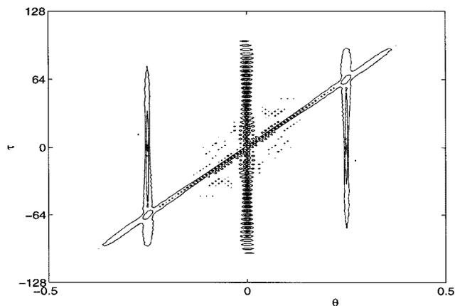
Fig. 1. Ambiguity functions of the chirp signal and two sinusoidal signals.
